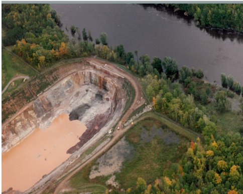
Following heavy rains the Flambeau River came within 20 horizontal and 4 vertical feet of spilling into the Flambeau mine pit. (Photo Bob Olsgard of Saron WI, 9.17.94)
